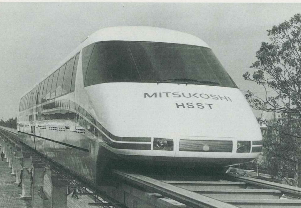
The HSST, a magnetically levitated train now officially approved for passenger transportation
