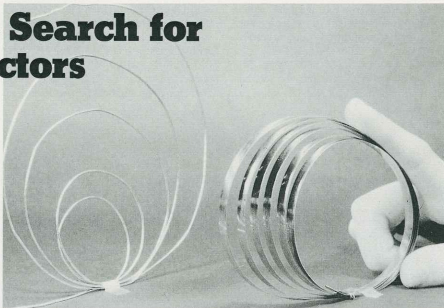
Superconductive wire of the type which was first discovered to be a higher-temperature superconductor.
